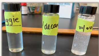
Figure 4: Treated and untreated solutions: veggie oil-based ferrofluid (left), decane-based ferrofluid (middle), and untreated microplastic solution (right).
