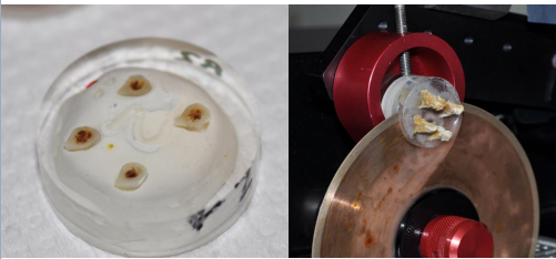
Figure 1: This is the epoxy puck with four bone samples embedded, cut and polished.
