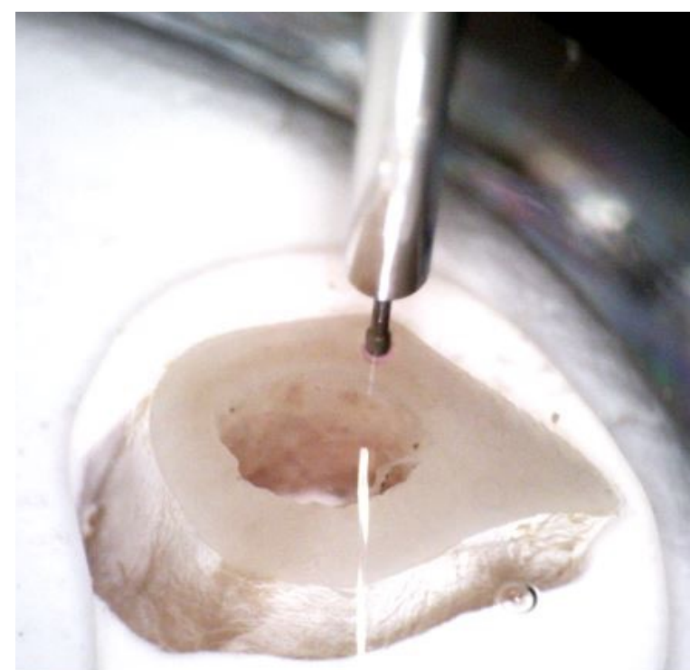
Figure 3: Photo taken with the dino-lite of micro-indenter tip and rat bone.
