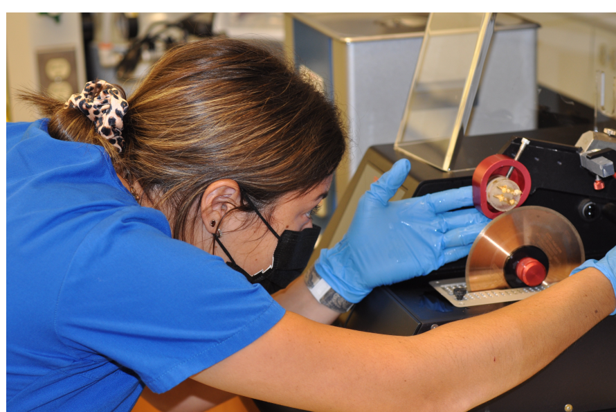
Figure 1,2: Photos taken during the process of cutting the bone pucks with the diamond saw.
