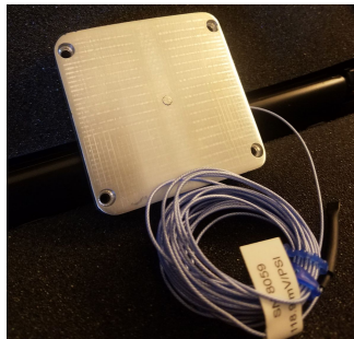
Modified port window with sensor installed
